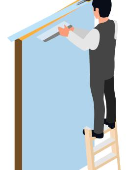
TRIM OFF ALL EXCESS WALLPAPER. USE A METAL PAINT EDGER OR BROAD KNIFE AND A **RAZOR KNIFE TO GET CLEAN EDGE. A FRESH BLADE SHOULD BE USED ON EACH CUT** FOR BETTER RESULT.
