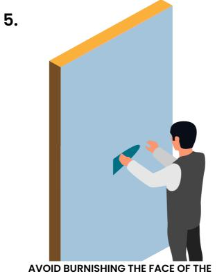
MATERIAL. USE A WALLCOVERING BRUSH OR A PLASTIC SCRAPER TO SMOOTH THE WALLPAPER ONTO THE WALL.
